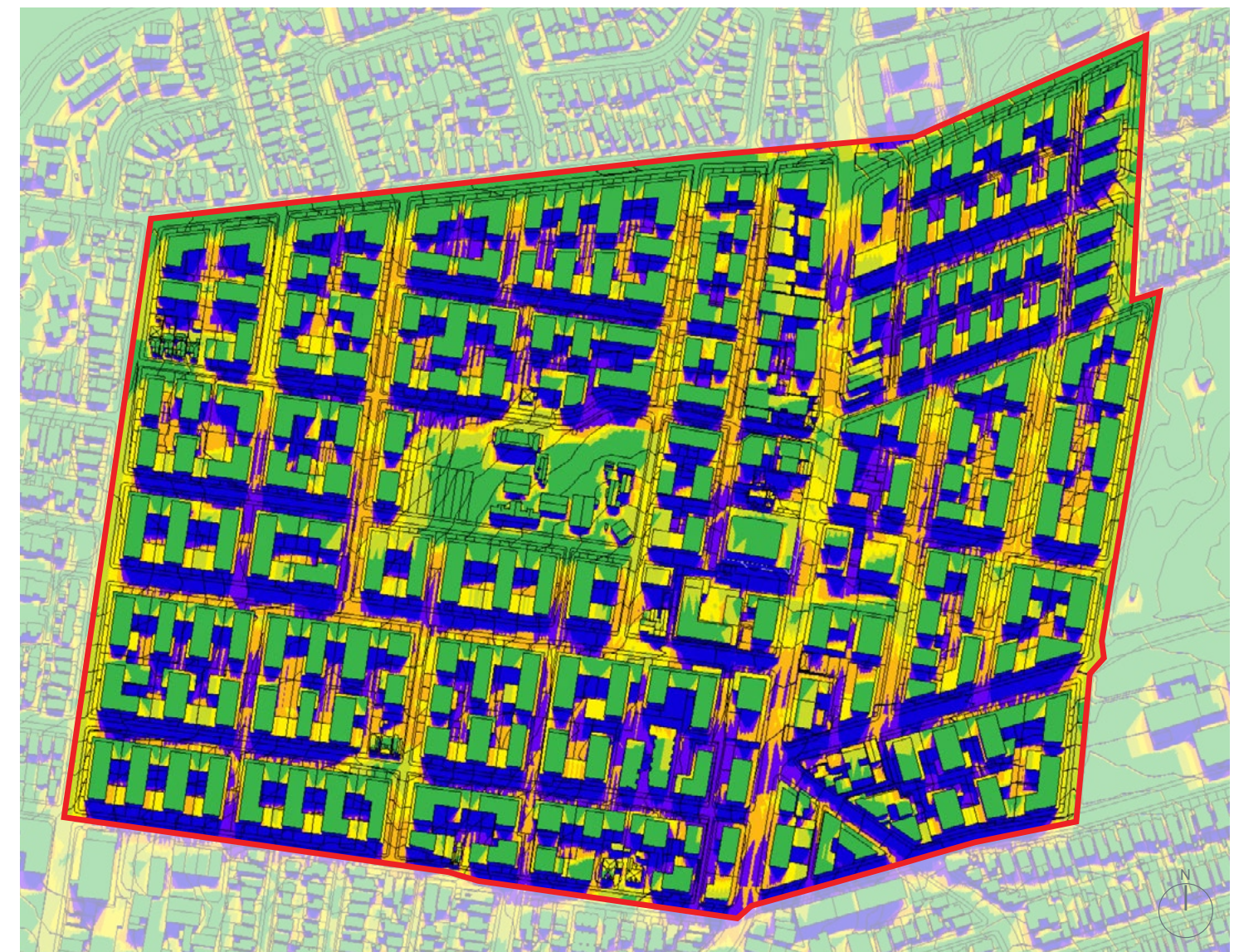
Figure 79 Solar access duration in mid-winter (June 21) between 9am and 3pm
