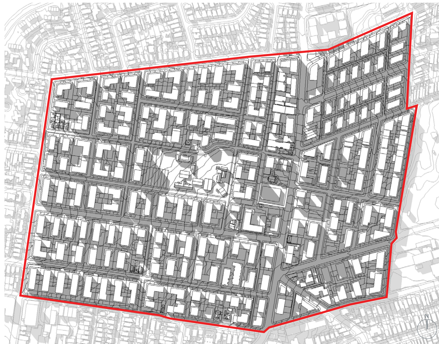
Figure 78 Shadow Diagram 21 June - 3pm
